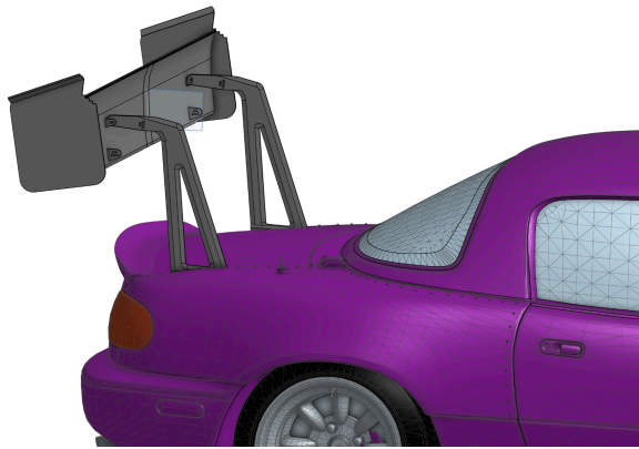
Figure 11: Full rendering with wing folded down, showing increased clearance and trunk access. 3D vehicle model courtesy of antoineallardchoquette via Sketchfab.
