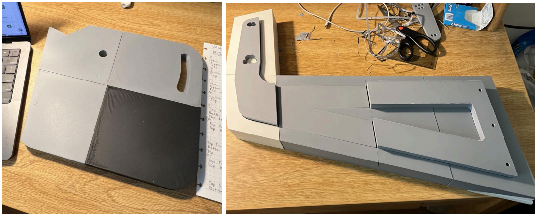
Figures 37 & 38: Completed 3D printed male endplate mold assembly (left) and completed 3D printed female and male pylon mold assemblies (right).
