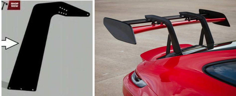
Figures 8 & 9: Outdated and bulky NLR wing pylon (left) and 992 Porsche 911 GT3RS swan neck wing, displaying modern, cutting-edge, trendy pylons (right)[2].
