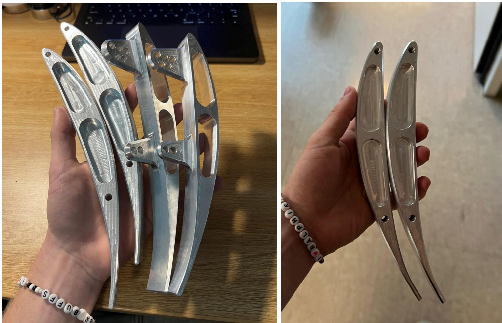
Figures 39 & 40: Freshly machined 6061 aluminum internal mounting and finished and tapped edge ribs.
